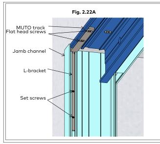
2.22.1 Use a plumb line to verify that the jamb channel is square to the horizontal track.
