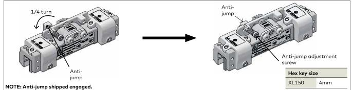
2.31.1 Disengage the anti-jump on roller carrier.
