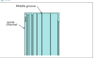
2.8.4 Jamb channel mounting holes: 1) Locate first mounting hole 6 inches from top.
