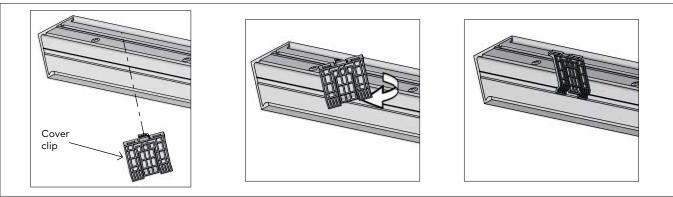
2.40.1 Insert cover clips into track. (One clip per foot)
