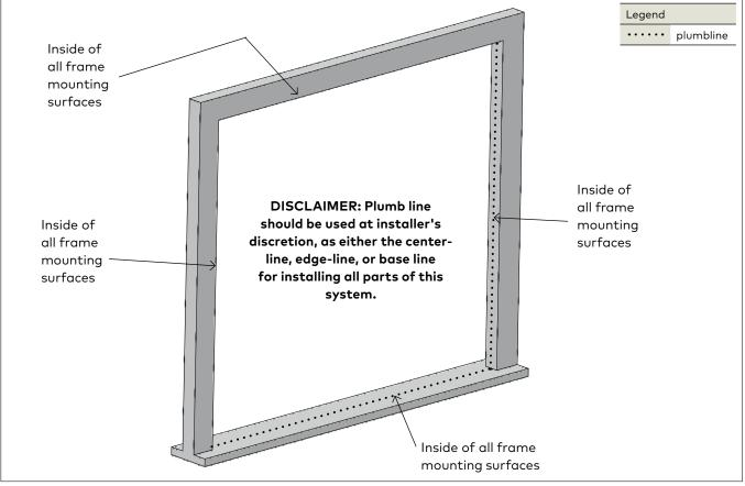
2.1.1 Mark a plumb line around the entire inside perimeter of the frame.
