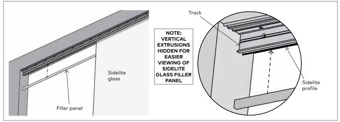
2.43.1 Fit filler panel into gap of the empty door panel section in sidelite profile.
