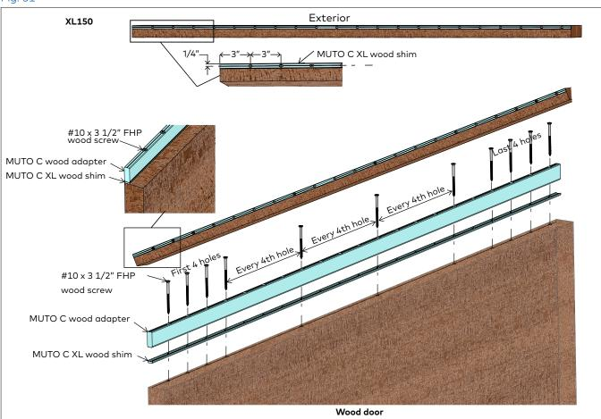
Install wood adapter and wood shim on top of wood door.
