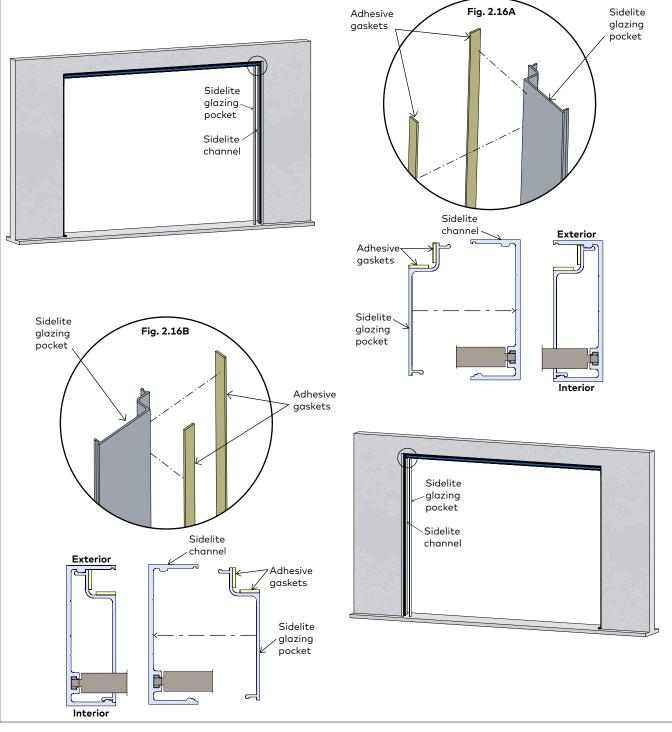
2.16.1 Measure and cut glazing pocket to appropriate length, if necessary.
