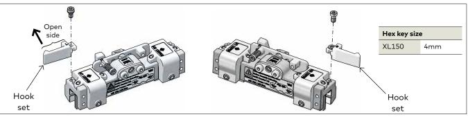
2.25.1 With rollers facing away from the installer, determine which roller will be leading and which will be trailing. 2.25.2 Secure hook onto roller with open side facing away from the installer.
