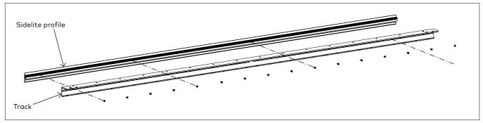
2.4.1 Align edge of sidelite profile with track extrusion.
